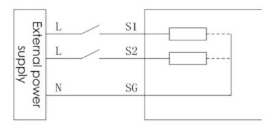
In general, when the external node is closed on, SPM32 LCD corresponding status input channel is ON (●), internal set to 1.
