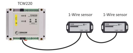
"Star" topology can be used only as a last resort for up to 4 sensors and total cable length up to 10 meters:
