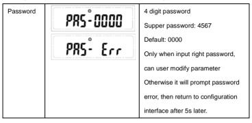
Note 1: Only in configuration interface, can user enter into password input interface after press ← >3s. Then LCD will display PR5 0000, the farthest right "0" flashing, customer can press ♠ to modify flashing digit (circle display from 0~9) and press ← to move cursor.
